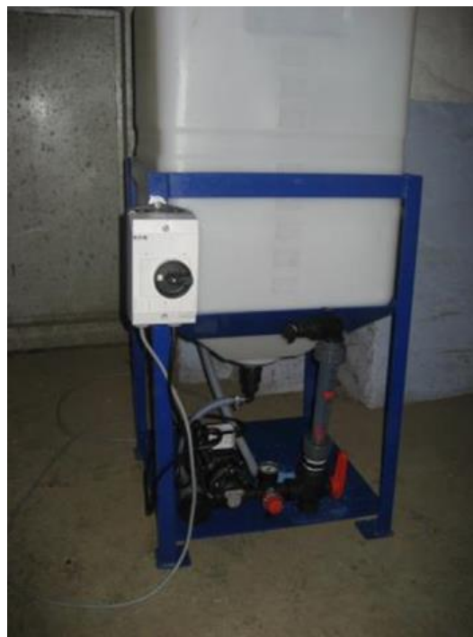
German K-Obiol applicator and spray drift arrestor
