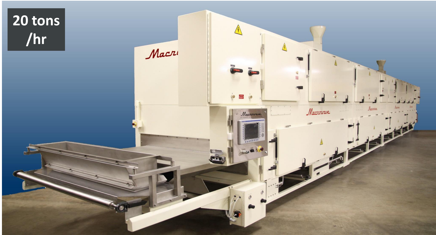
Large 400 kW Pasteurization System Example
