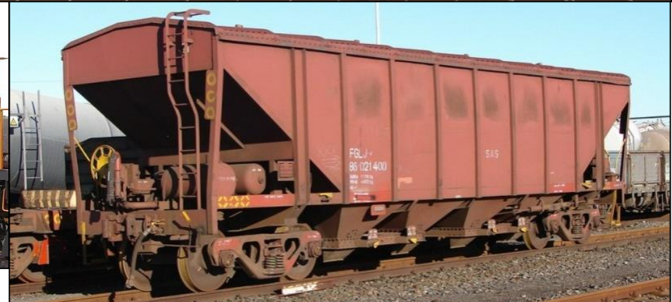
44 t payload capacity-3 or 4 hoppers
