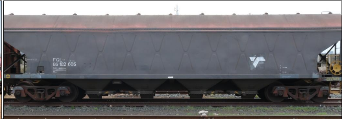
60 t payload capacity-4 hoppers
