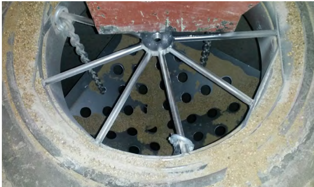
The silo umbrella concept in action. An umbrella with a flow rate of 120t/h was installed inside a concrete bin to reduce malt breakage. (Photograph: Johan Olivier)
