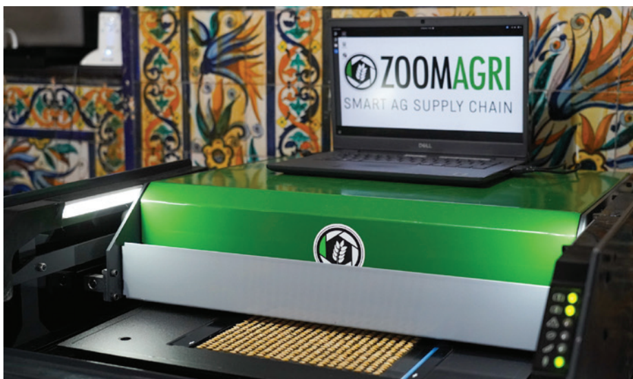
ZoomAgriSpex to determine the physical quality and classification of grains and oilseeds.
