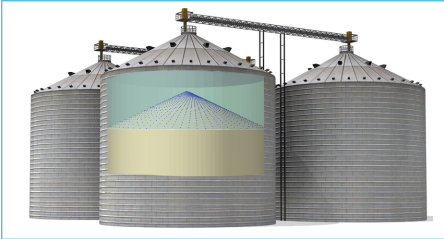
Figure 1: A representation showing how Ronin's laser technology generates information pertaining to the exact grain volume inside a silo.
