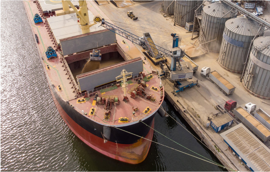
World norms for receiving and loading grain vary between 10 000 and 15 000 tons per day, with some able to load up to 25 000 tons per day.
