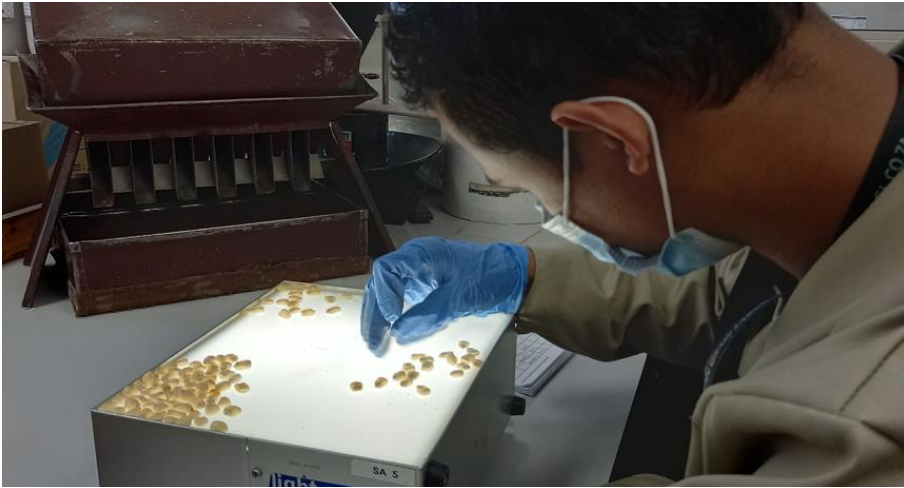
Determining the percentage of maize kernels with stress cracks on a light viewing box in the grain laboratory.
