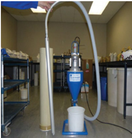
The Vac-A sampler double pneumatic suction probe (Seedburow) and 200mm diameter cylindrical plastic container with the grain or oilseed sample.
