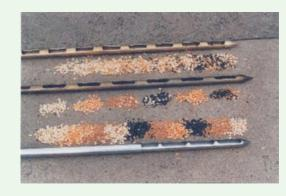
Double pneumatic suction probe (VAC-A-Pneumatic sampler, imported - USA)
