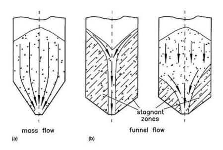
A function of bin geometry and bin hopper characteristics
