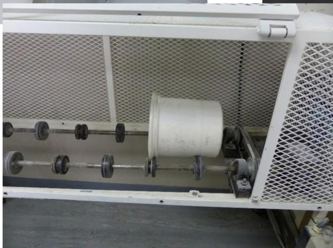
**Mixing of milled sample for 90 min to ensure homogeneity of the sample**
