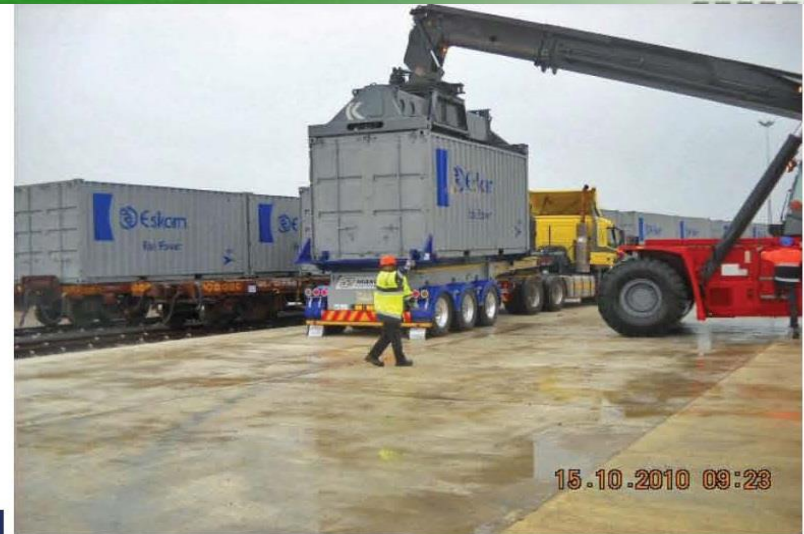
Container transferred by reach Stacker to Rear Tipping vehicle or Rail Wagon
